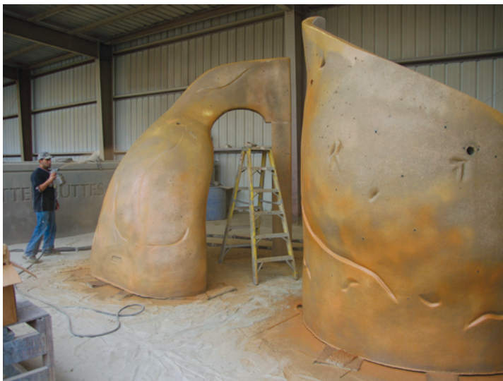
A UNIVERSAL EMPLOYEE ADDS COLOR TO A PRECAST ROCK WALL.
