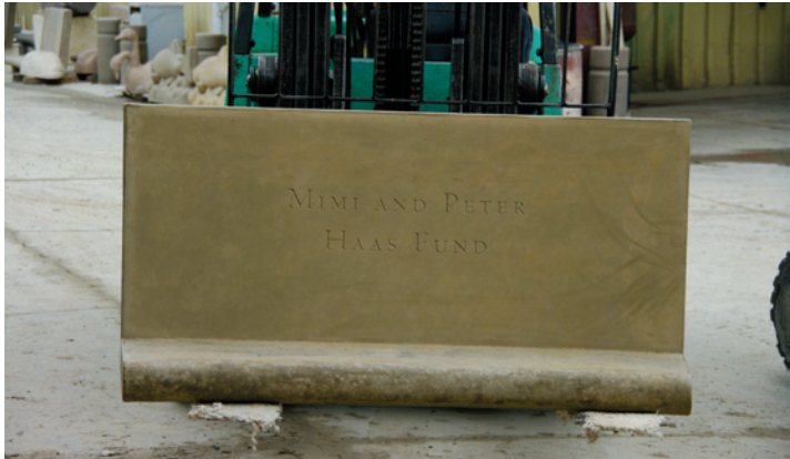
A BENCH WITH INSET LETTERING ON ITS WAY TO CURING AFTER BEING STRIPPED FROM ITS FORM.
