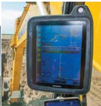
Komatsu's *intelligent* Machine Control excavators feature semi-automatic operation that goes beyond traditional indicate-only systems. Once target elevation is reached, the system limits the machine from digging deeper, eliminating overexcavation and the need for expensive fill material.
