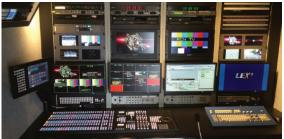
Applied Video Technology, Inc. (AVT) was contracted to provide equipment, design services and installation to implement a full HD Mobile Production Truck for RCN Cable TV in Bath, PA. The AVT sales and engineering team worked closely with RCN engineers throughout the course of the project to design the complete renovation of the truck. Features include an all new custom interior, electrical wiring, audio and video wiring and updated HD production equipment including
