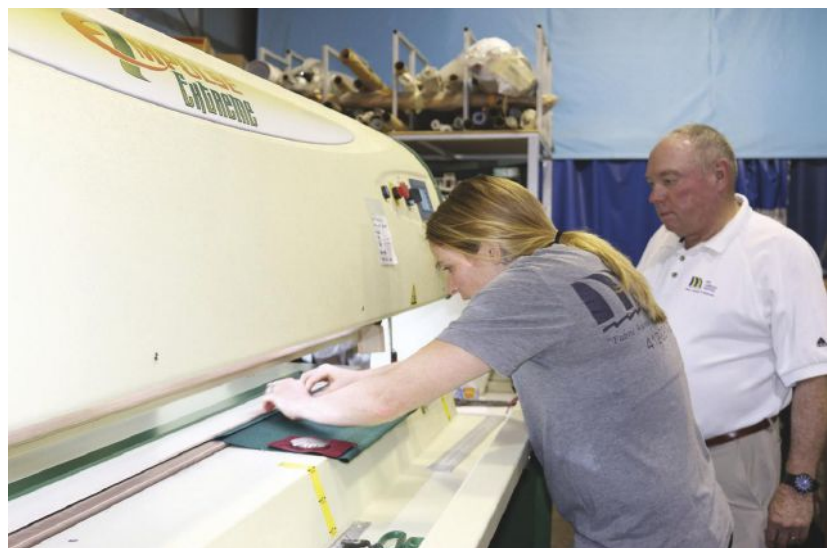
Cristin Conlon (left) and Bob Campbell use an impulse fabric welder to seal fabric seams, which utilizes high pressure and heat for a quality seal.
