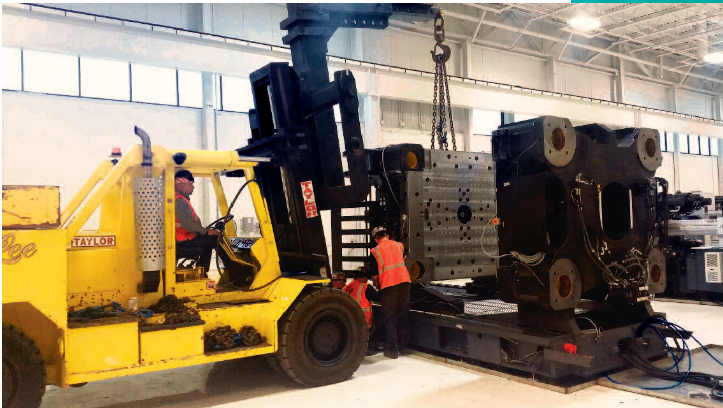
Lee Riggers are assembling the clamp on a 1300T Haitian Injection Molding Machine.
