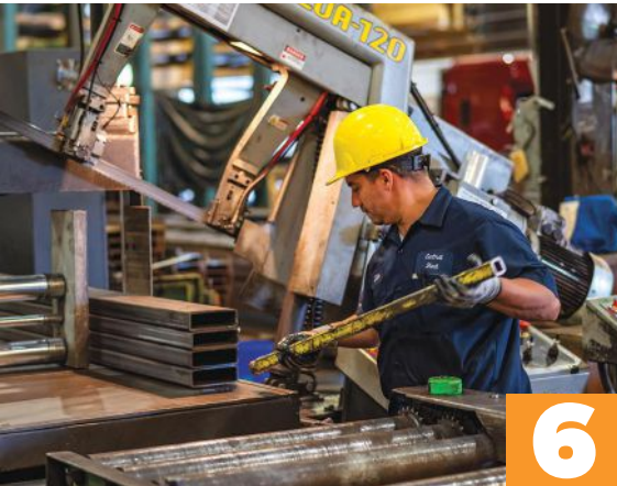
Machine Operator Julio Lazo of Central Steel Supply Company, Inc. evens off the ends of a steel bar in preparation for cutting.
