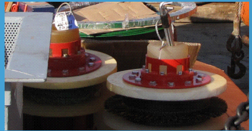
Pig for cleaning the pipeline.
