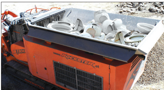
A Rockster R1000 impact crusher recycles porcelain toilets.
