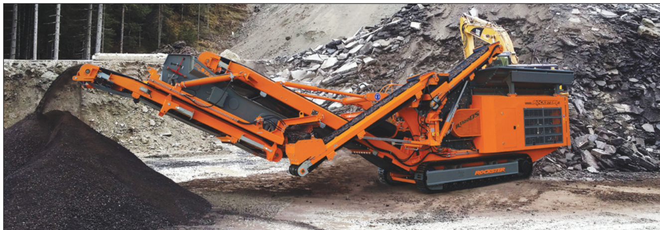
A Rockster R1100DS impact crusher recycles RAP for reuse as adjunct for new asphalt.
