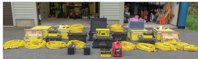
Geoscy LLC can handle large jobs with its extensive electrical resistivity imaging (ERI) equipment.
