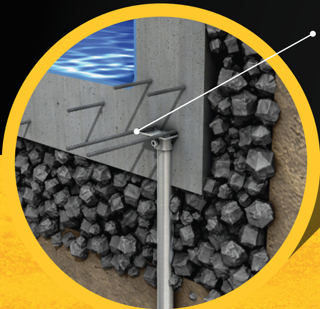
PILE HEAD WITH REBAR
