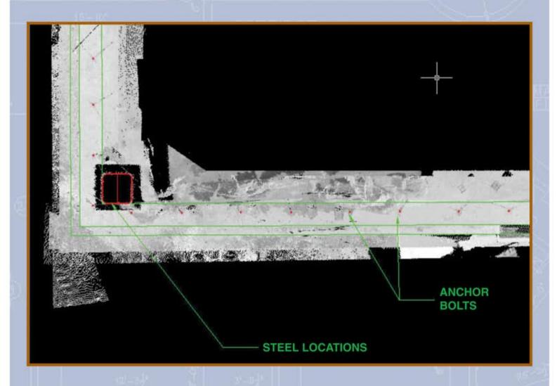
Scans files are processed in CAD software. A "slice" is taken through the 3D model and a section created one inch above concrete, where the bolt is "straight."
