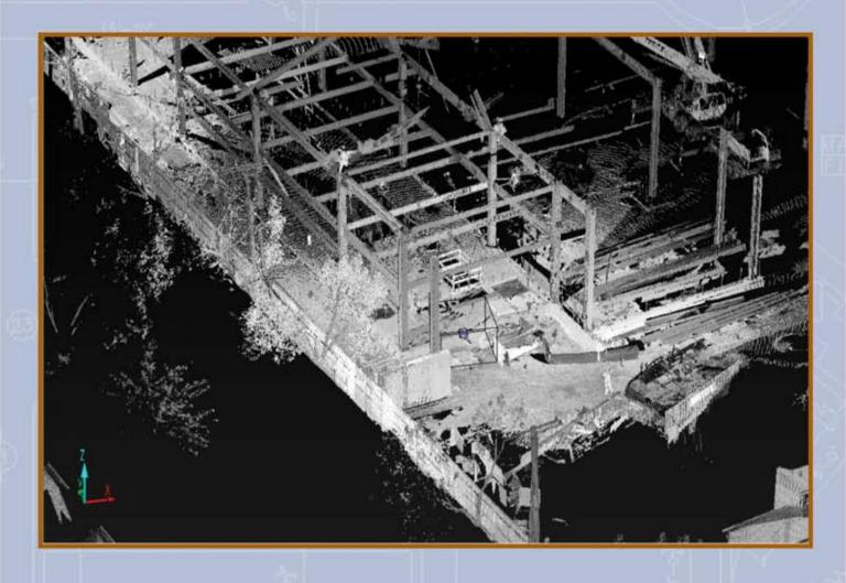
All scans are aligned to create comprehensive digital map of the construction site that can be measured or used as a foundation to create a BIM document for coordination of trades.
