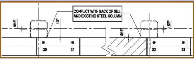
While the scope of work included only producing accurate as-built drawings of the anchor bolts, a thorough inspection of the 3D scans showed that the structural steel was placed incorrectly. An error normally not detected until the stone setter mobilized and the material was onsite.
