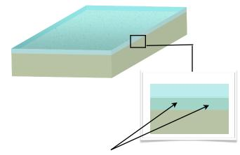
HP Spartacote<sup>TM</sup> effectively absorbing into ("wetting") the substrate.
