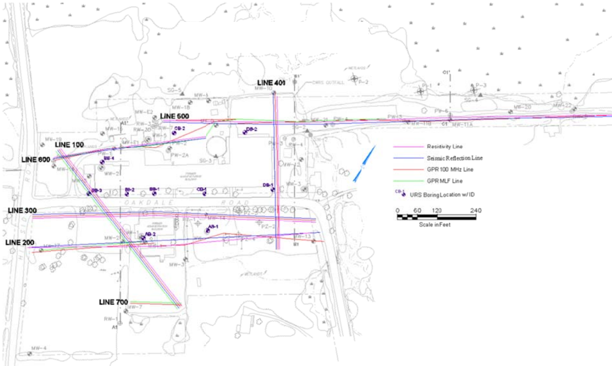
Figure 3: Geophysical survey and borehole survey locations.
