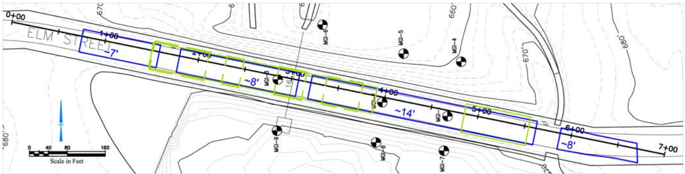
Figure 6: AutoCAD plot showing the locations of GPR (dark blue) and MASW (green) anomalies.
