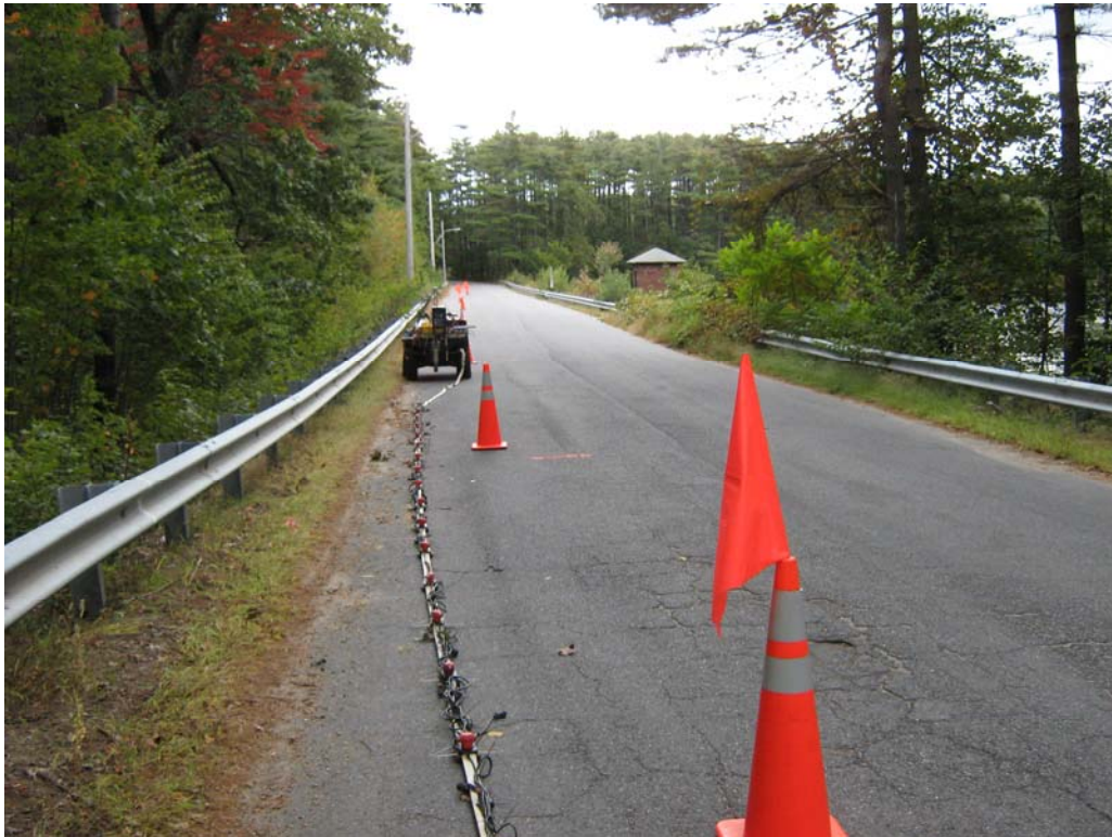
Figure 5: MASW seismic line setup showing land streamer array with ATV.
