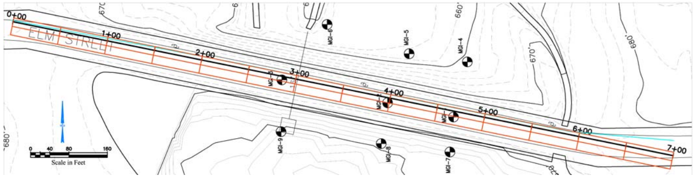
Figure 2: Topographic map of earthen dam and surrounding area showing locations of GPR (red) and MASW (light blue) traverses.
