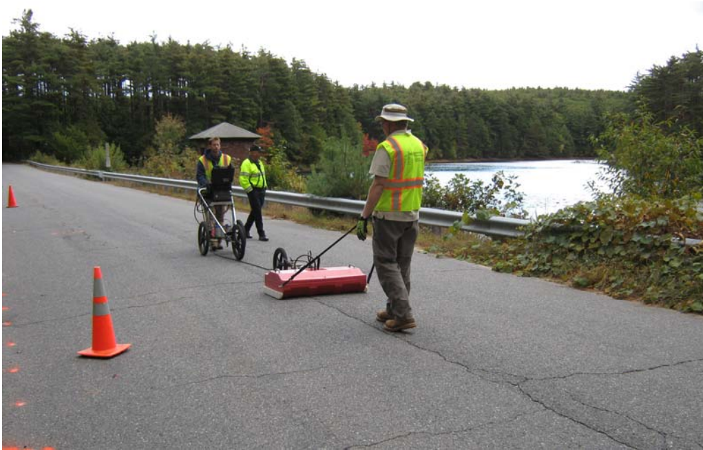
Figure 3: GPR data collection using the 100-MHz monostatic antenna in survey wheel mode.
