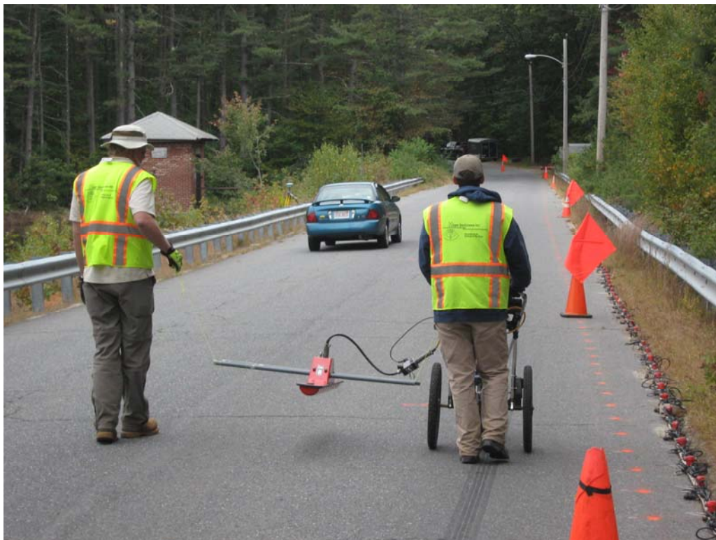
Figure 4: GPR data collection using the 70-MHz bistatic antenna in survey wheel mode.
