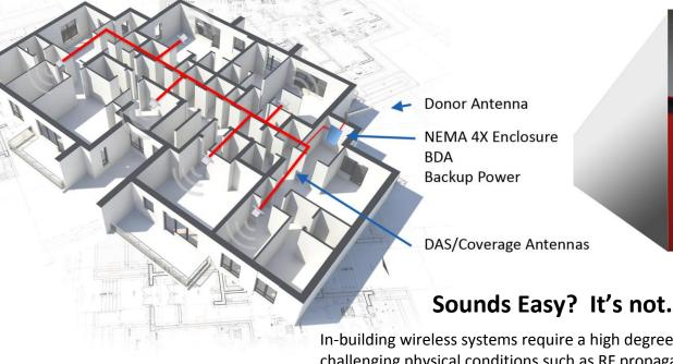
In-building wireless systems require a high degree of design and implementation expertise to meet the many challenging physical conditions such as RF propagation intricacies, networking elements and carrier requirements. An improperly designed or installed system can contribute to communication problems in emergency situations, as well as cause interference to other systems that can result in legal actions and substantial fines.
