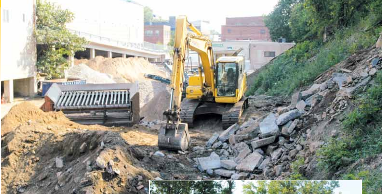
(Above) Metro Green uses its Komatsu PC160LC-7 excavator at a jobsite and (right) when loading its Metso LT95 jaw crusher.
